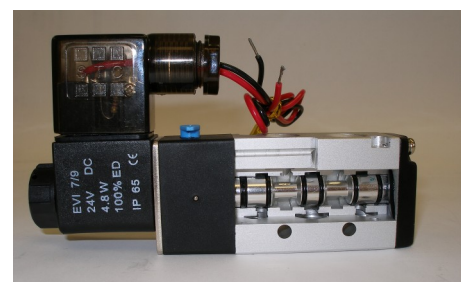
Figure 2: 4-way valve with cutout, showing piston.
